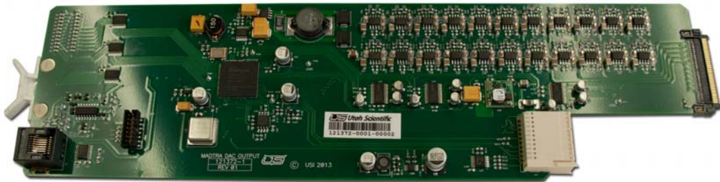
Figure 1-9. DAC Audio Output (121372-1)
